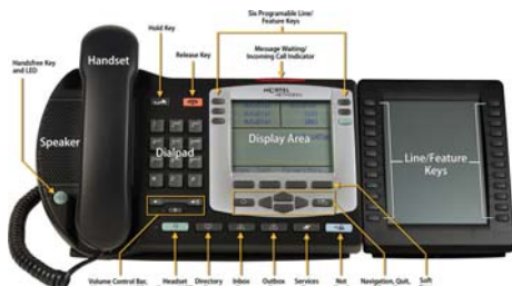
Diagram 7—Key Expansion Module The IP Phone 2004 supports the use of two Key Expansion Modules (KEMs) for a maximum of 50 programmable keys.
